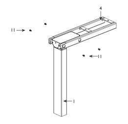
The Frame End-CB (part 3) should be placed on the side of the desk where you plan to mount the Control Box (part 7) and the Handset (part 8).
